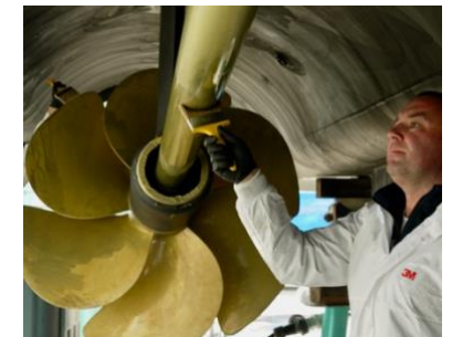
Application du "Clear Coat"
