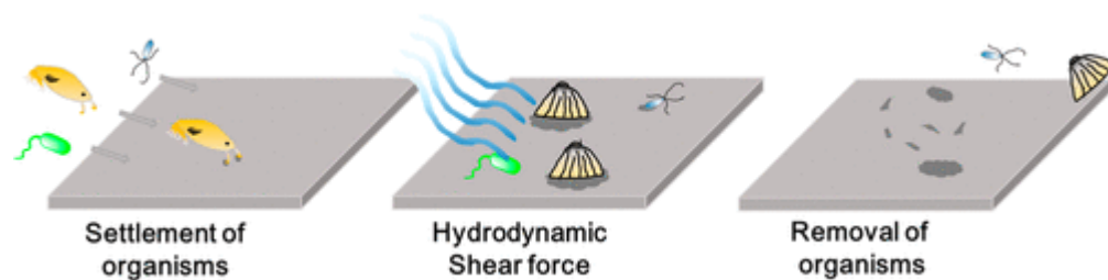
Figure 1. Schematic of fouling-release coatings.
