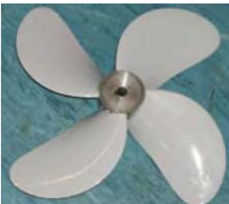
Figure 10: The model propeller with mated blades.
