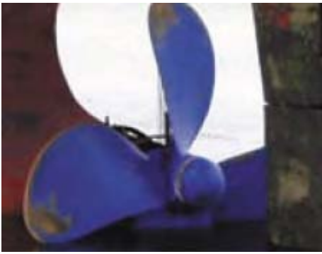
Figure 18: The full scale propeller after 37 months of service
