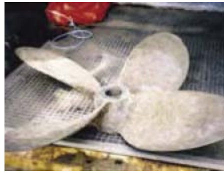
Figure 4: The propeller of 'Bernicia' after 14 months in service before coating. Hard shell fouling is present to half the blade radius.
