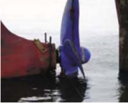
Figure 19: The back of the full scale propeller after 37 months of service.
