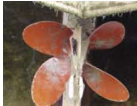
Figure 5: The propeller of 'Bernicia' after 12 months in service after coating. 95% of the coating is intact, except some detachment of the blade edges. Light slime fouling is present in the inner half of the blades (grey material in the red coating is the dried bio film). This could be easily removed by hand or with a damp cloth.
