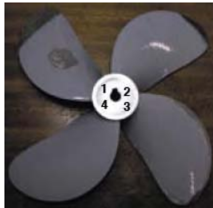
Figure 14: Damage Scenario 2 [view from the back].
