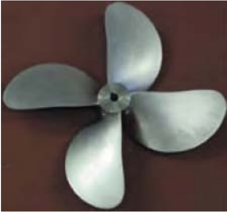
Figure 9: The model propeller with uncoated blades.
