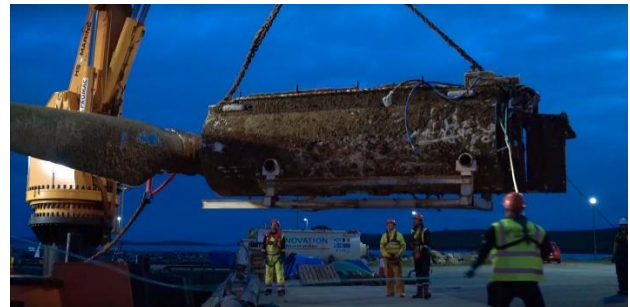
Figure 1 Fouled turbine by NOVA Innovation
