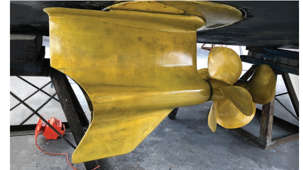
PropOne applied to a Volvo IPS unit
